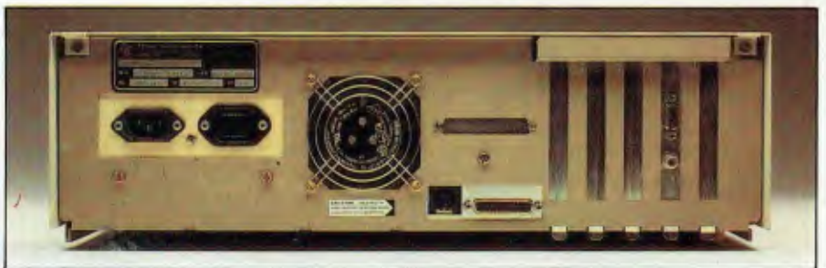
A parallel printer port is standard instead of RS232.
